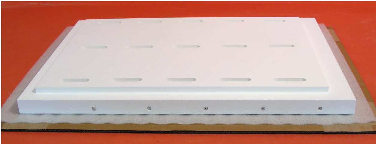
Typical roof panel with embedded reinforcing rods.
