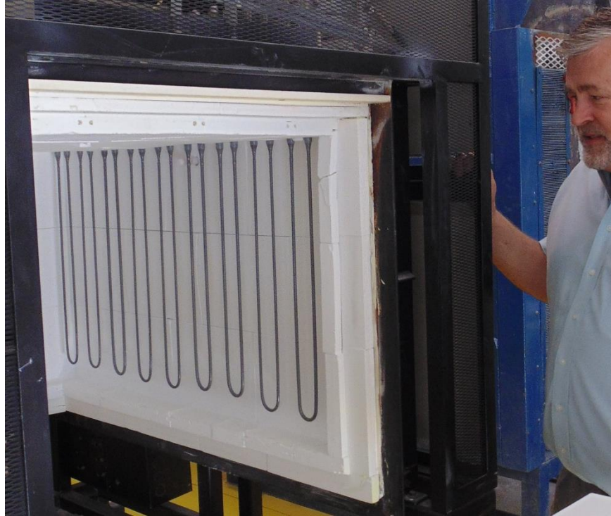
Pictured above is a 1700°C Shuttle Kiln. This kiln uses the FIM technology and is cycled from room temperature to 1700°C and back in 38 hours.
