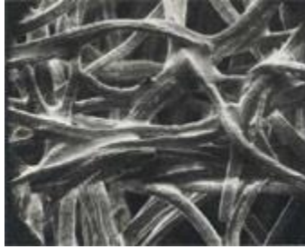
This 30 pcf density ceramic insulation shows a typical structure with open porosity.
