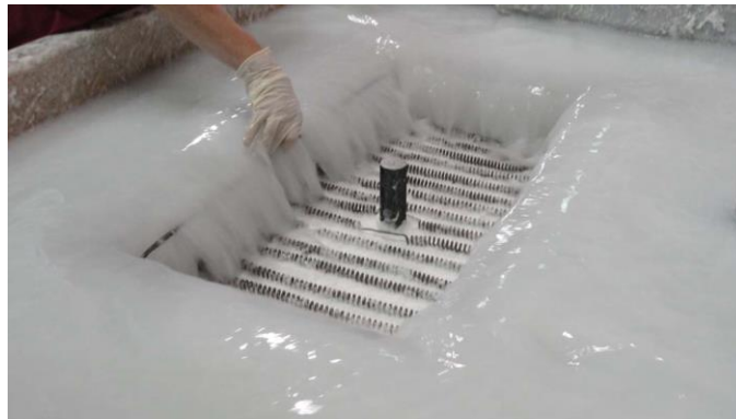
Producing vacuum formed ceramic fiber insulated heater.
