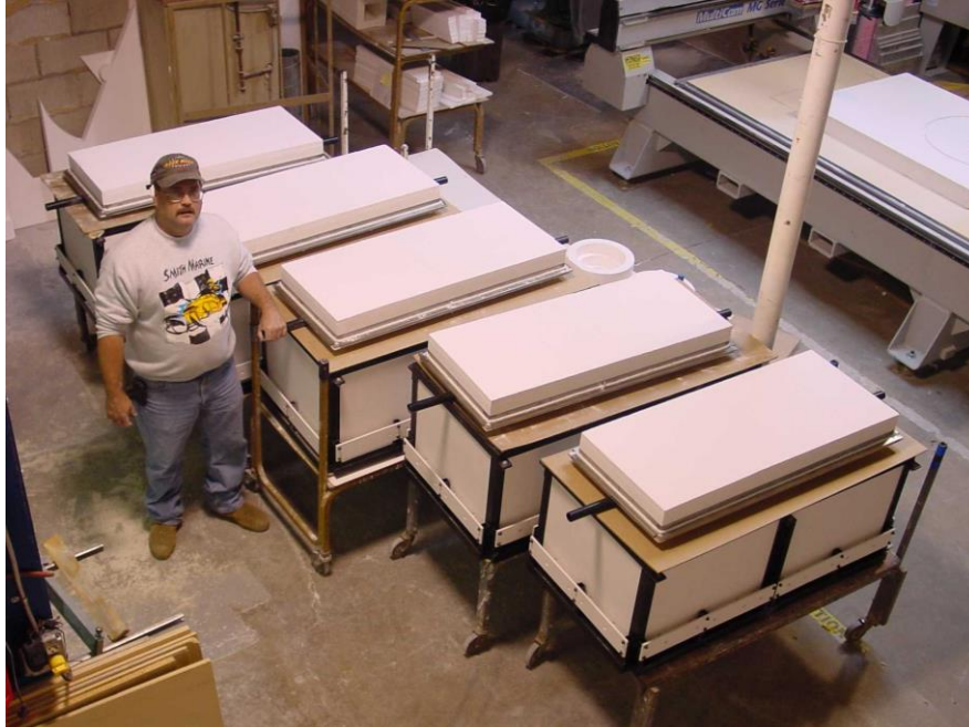
The Furnace Chambers shown above are used in the sintering of PTC Thermistors who's dielectric properties can only be achieved through extremely fast thermal cycling.
