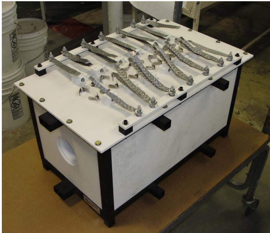
This lab-scale 1700°C rated Horizontal Tube Furnace Insulation Module utilizes reinforcing rods embedded in its roof. Its relatively small size and gradual heat up/cool duty cycle permit the use of Non-reinforced walls and floor insulation panels.
