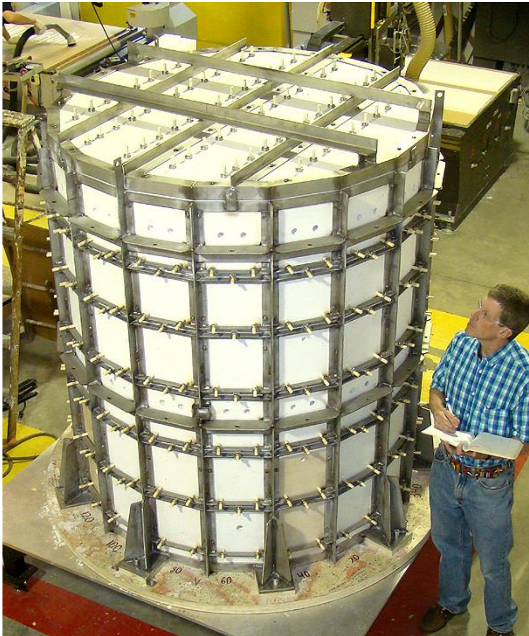
The 1700°C Furnace Insulation Module shown above utilizes the FIM technology.
